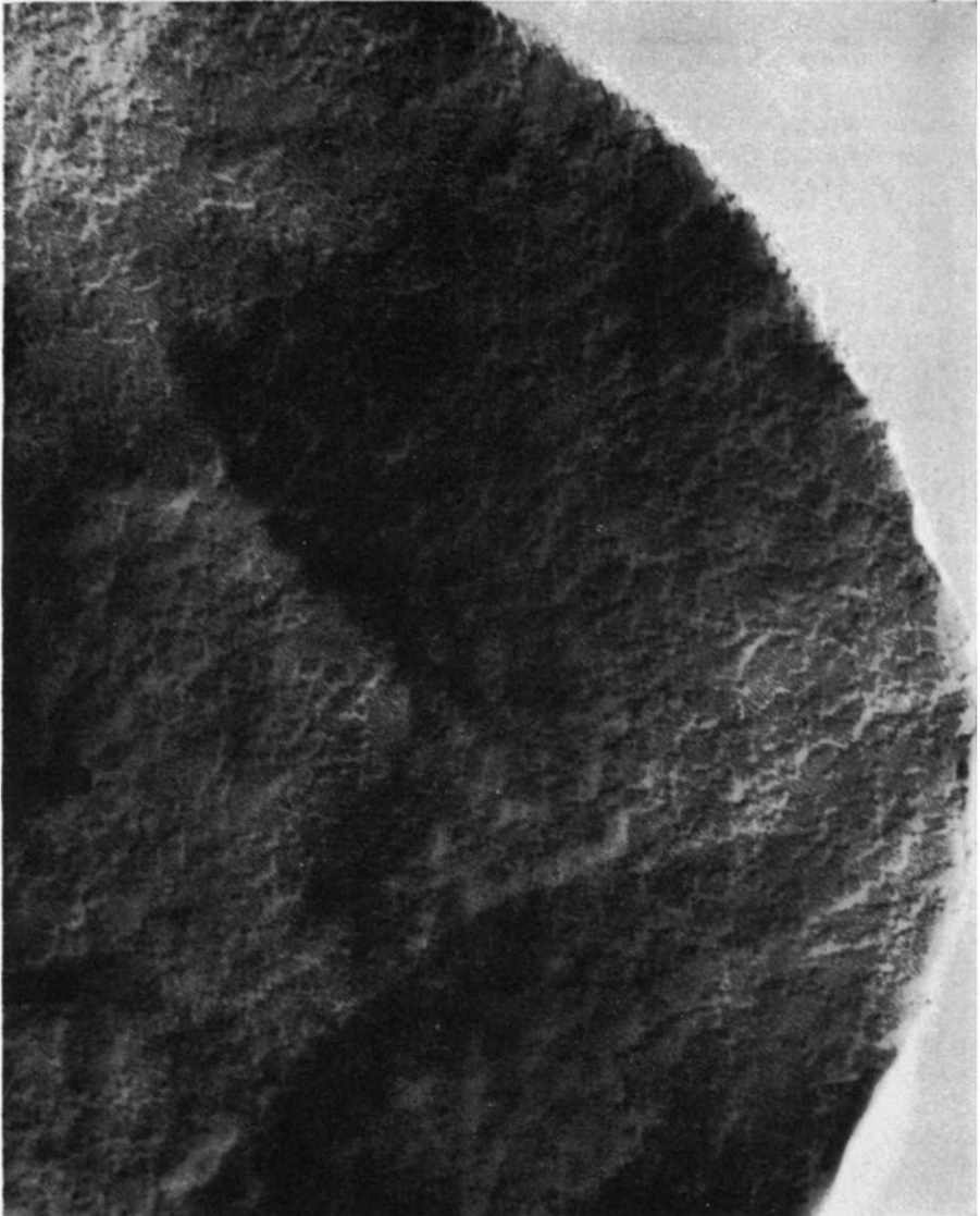
Figure 10 —Electron micrograph of part of a poly-4-methyl-pentene-1 crystal grown at 84°C from 0.070 per cent xylene solution shadowed as given in Figure 9 (Note 1 \mu spacer on LHS)
