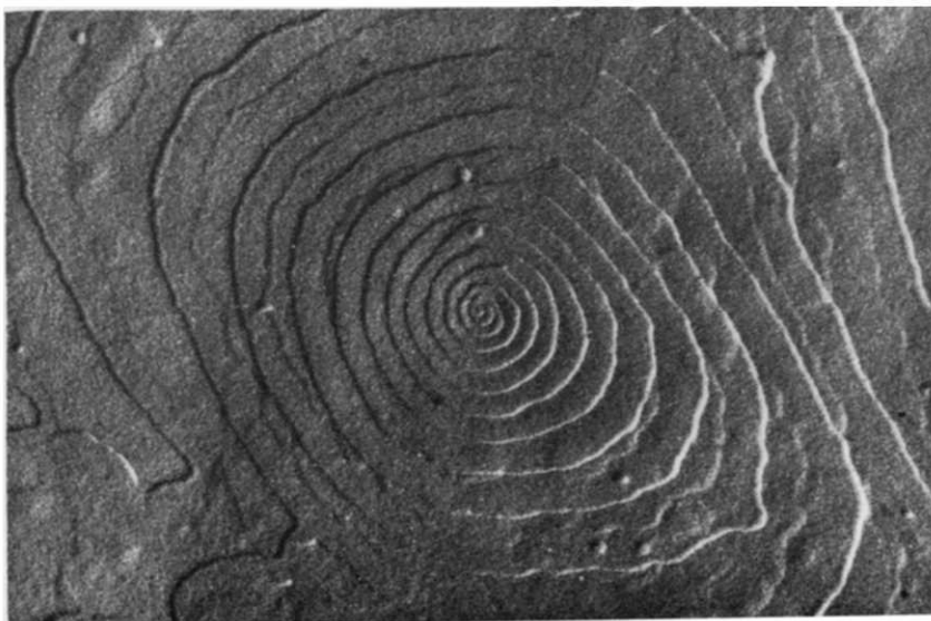
Figure 3 —Electron micrograph of shadowed surface replica of bulk crystallized polyethylene oxide crystallized at 50°C
