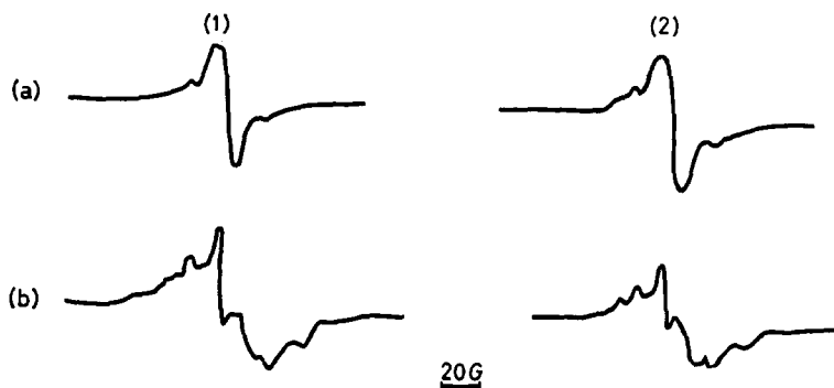
Figure 3—E.s.r. spectra of isotactic PMMA (3) irradiated and observed at 77°K: (a) as supplied by the manufacturer, (b) the same material purified. (1) Immediately after irradiation, (2) two weeks later
