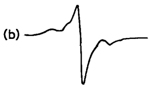
Figure 18 —E.s.r. spectra of PMA irradiated at 77°K and viewed at room temperature: (a) immediately on warming to room temperature, (b) 10 3 minutes later
