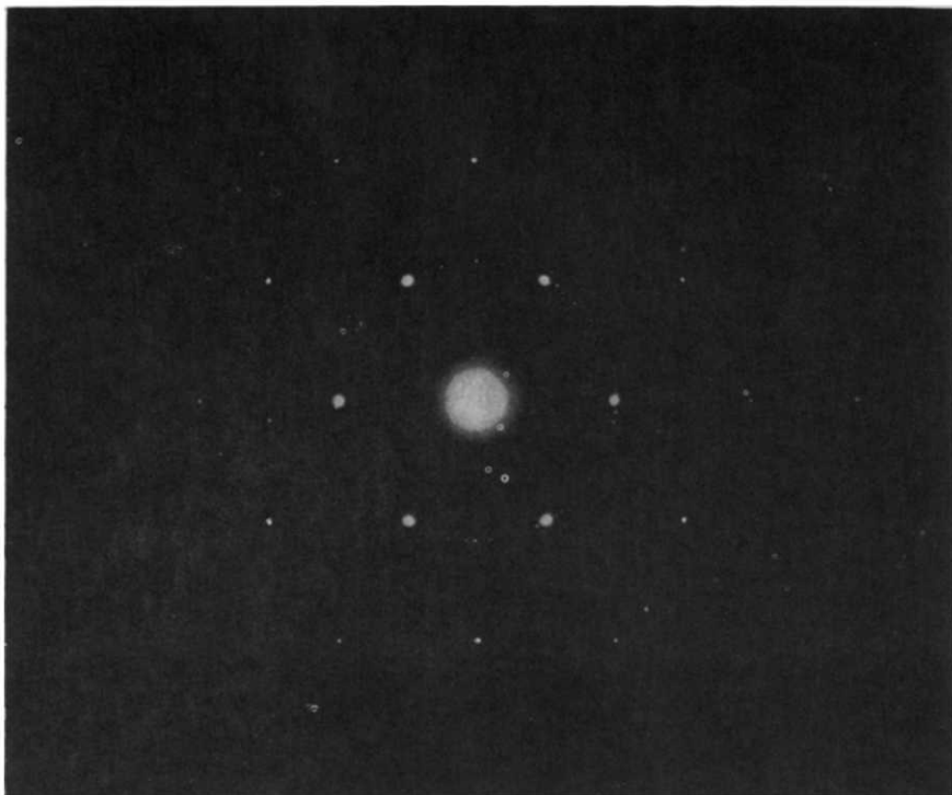
Figure 2 —An electron diffraction pattern from a POM crystal
