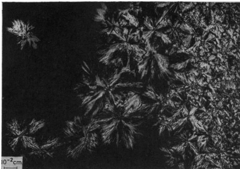
Figure 1 —Fraction 3 heated for 20 min at 200°C in form of film ca. 5 \mu thick, between glass cover slips. Crystallized at 128.0°C for six hours
