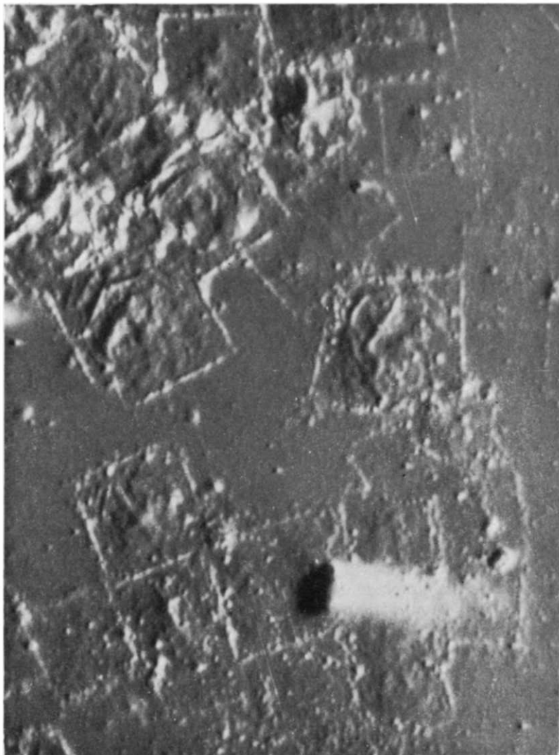
Figure 2 —Photomicrograph of a group of poly-4-methyl-pentene-1 crystals prepared as given in Figure 1 . Aluminium shadowed at \cot^{-1}4 . Magnification 1260X. Reproduced without reduction
